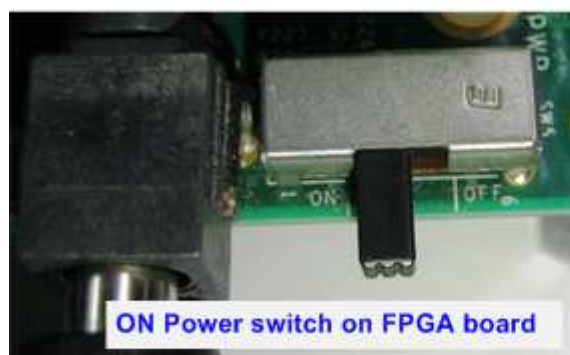
Figure 2-5 Power on FPGA and AB16 board on ArriaV GX Starter board.
