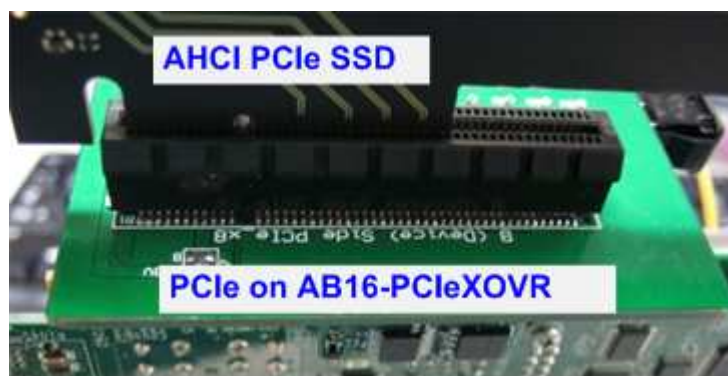
Figure 2-3 Connect AHCI PCIe SSD to AB16 board
