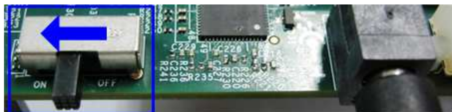
Figure 2-8 Power on ArriaV SoC board
