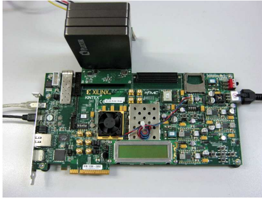
RAID evaluation on KC705 with 4 SSDs
