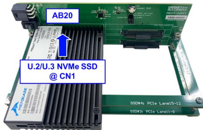
Figure 7 Connect U.2/U.3 NVMe SSD to CN1 of AB20
