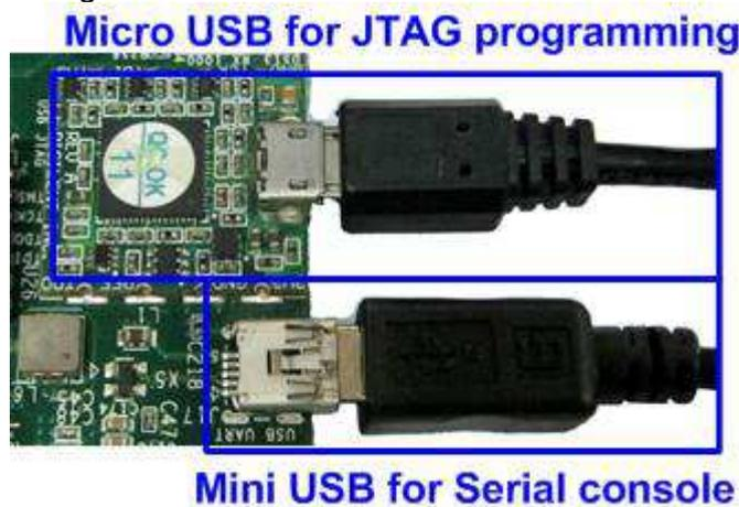
Figure 2-6 USB cable connection
