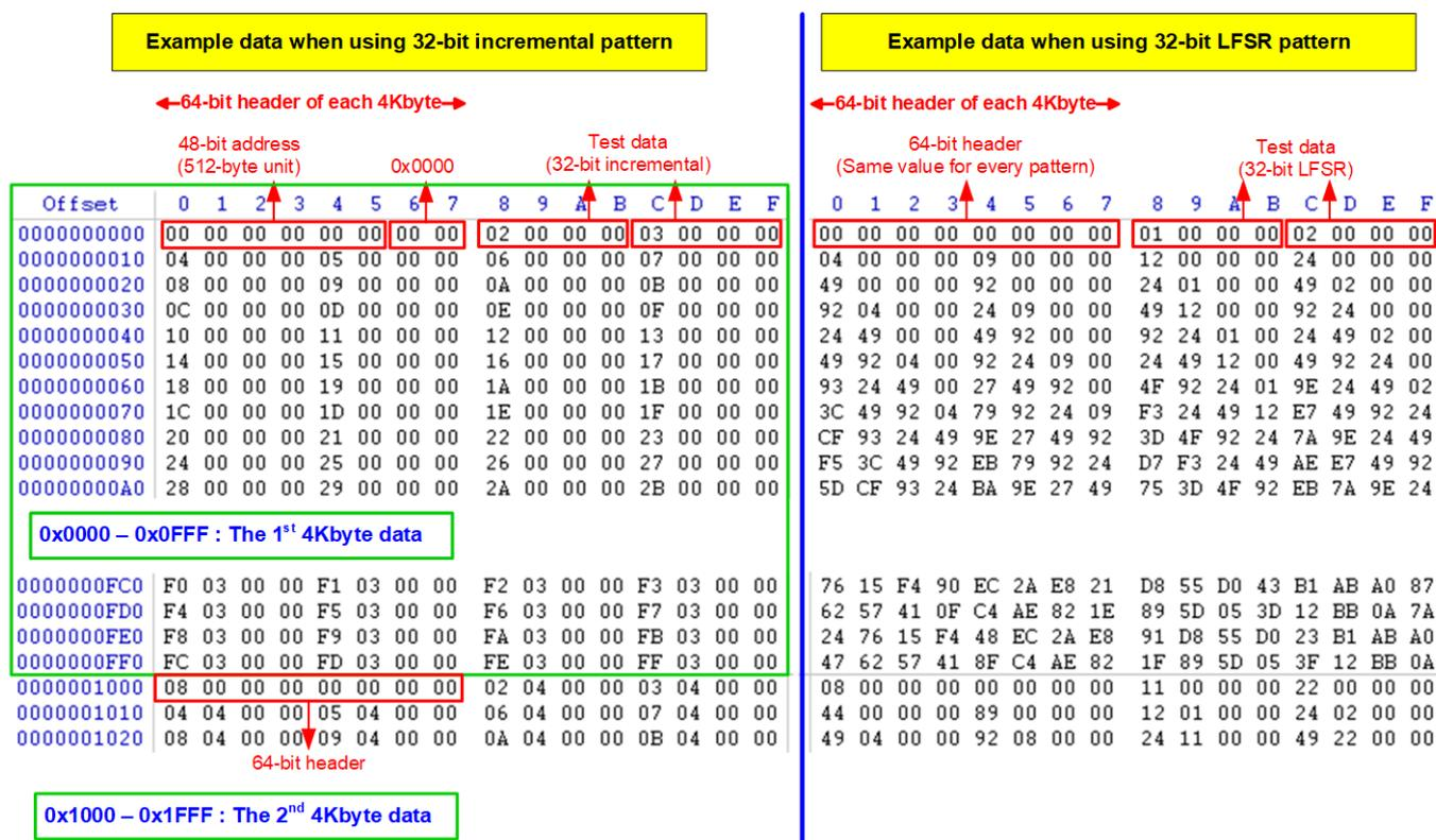
Figure 2-4 Example Test data of the 1<sup>st</sup> and 2<sup>nd</sup> 4Kbyte data by using incremental/LFSR pattern
