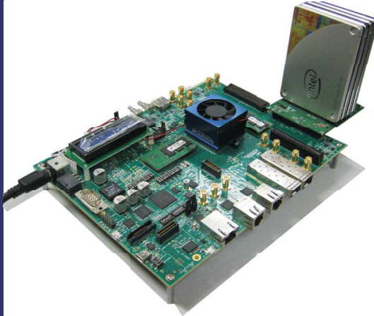
Evaluation on Intel®Arria® 10 SX FPGA Dev. Kit with AB09-FMCRAID + SATA3 SSD x 4ch RAID
