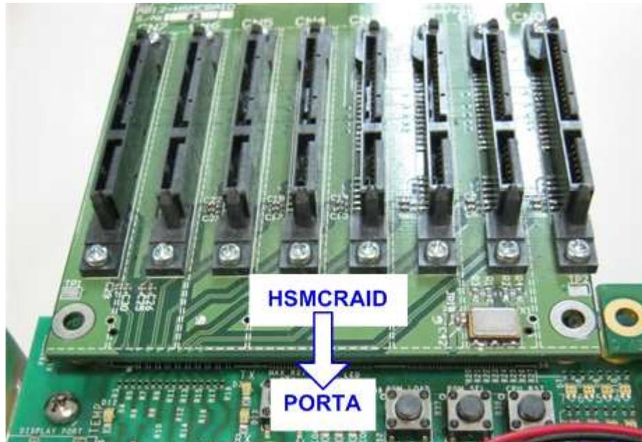
Figure 1-2 HSMCRAID Connection
