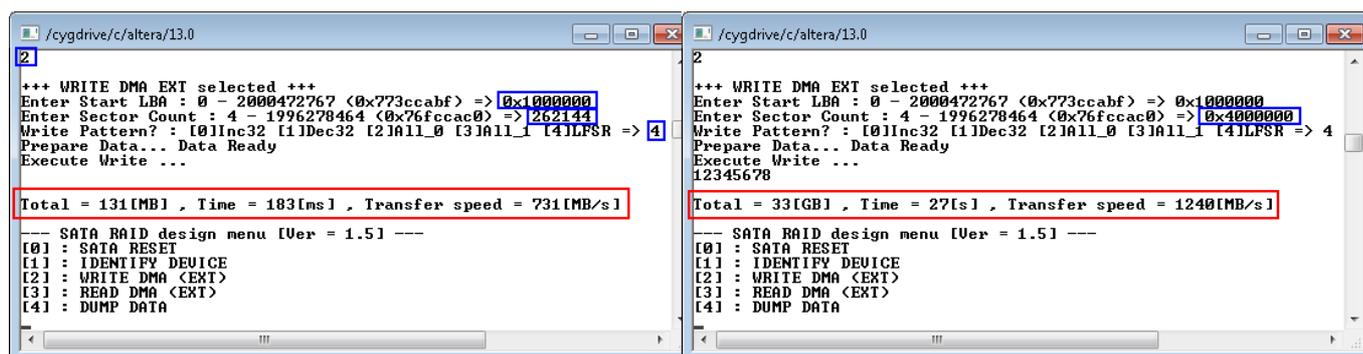
Figure 2-3 WRITE DMA (EXT) command input and output
