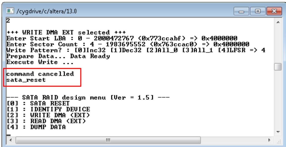
Figure 2-5 Write Operation cancelled from receiving input during operation
