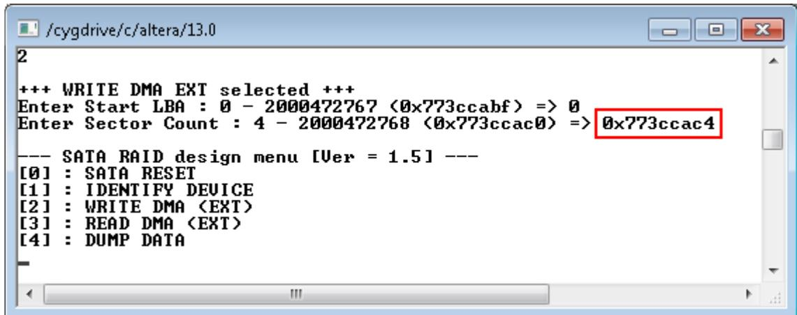
Figure 2-4 Write operation cancelled from error input
