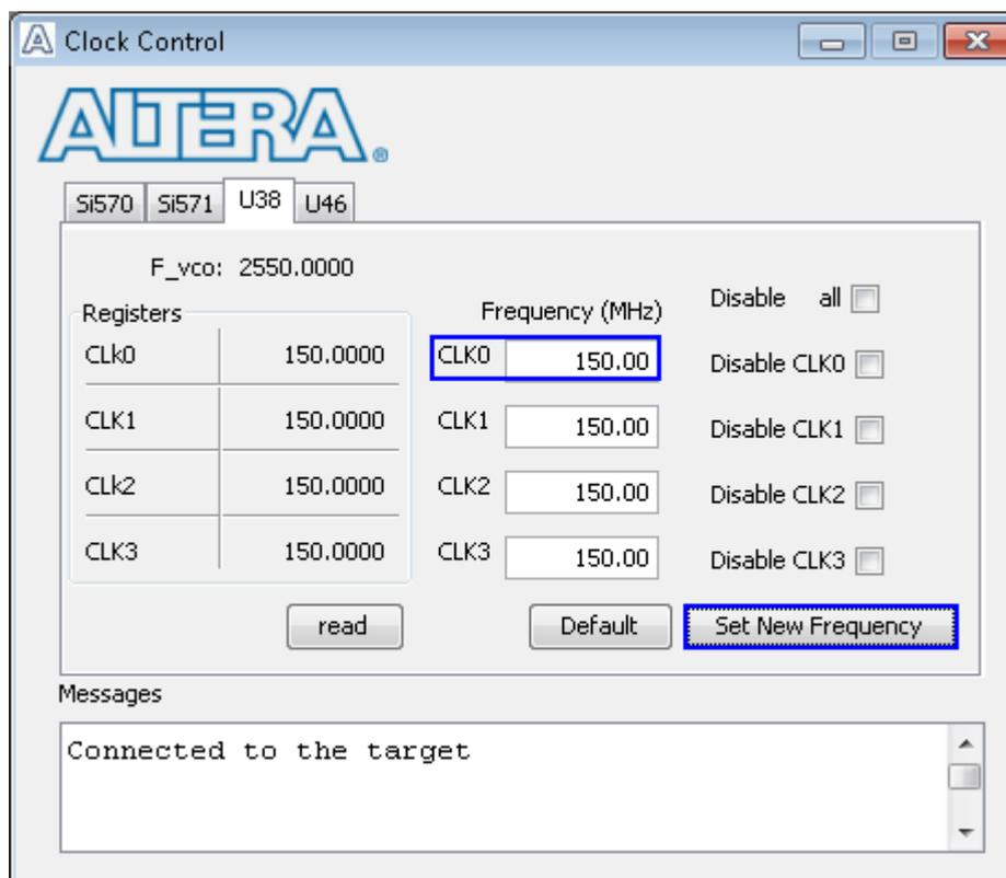
Figure 1-5 Set programmable clock = 150 MHz by Clock Control Application
