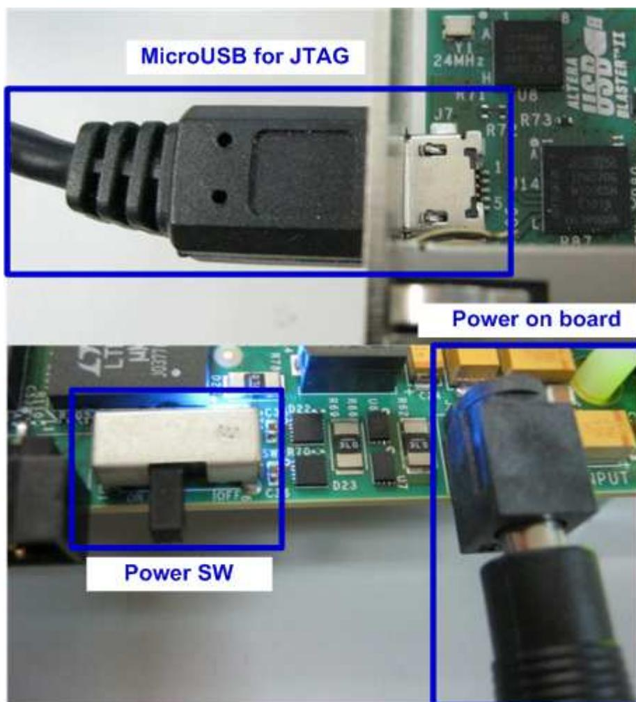
Figure 1-4 MicroUSB and Power Connection
