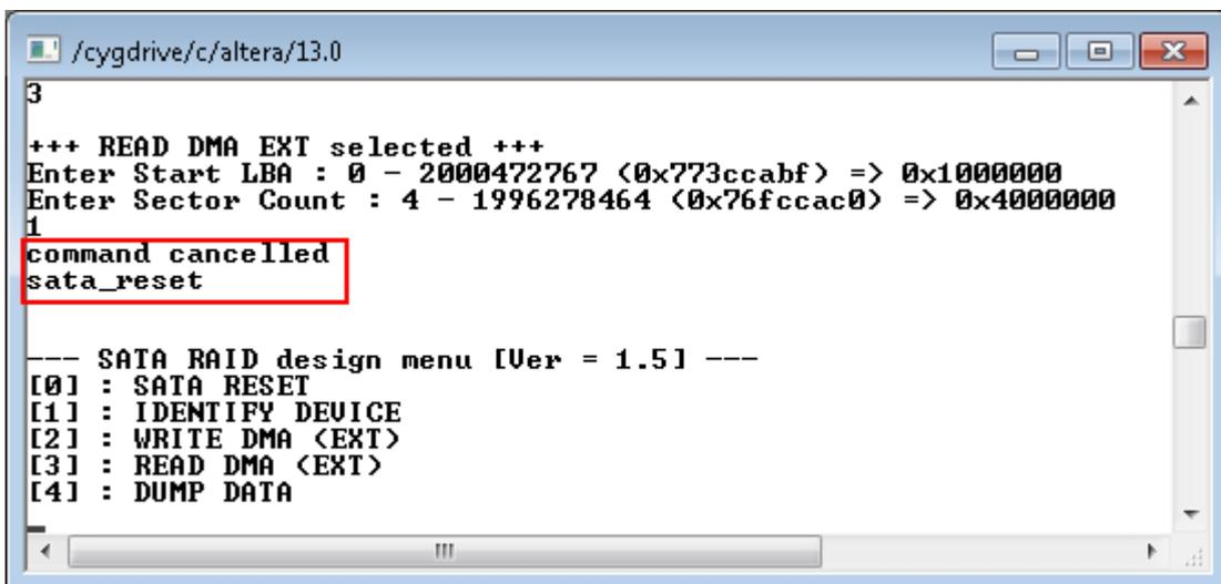
Figure 2-9 Read Operation cancelled from receiving input during operation
