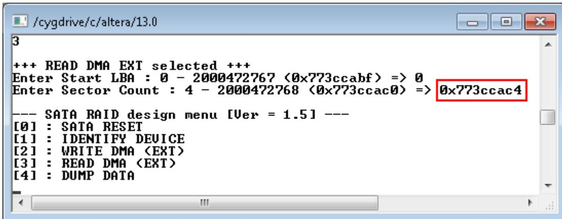
Figure 2-8 Read Operation cancelled from error input
