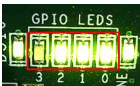
Figure 2-2 LED status after system set up complete
