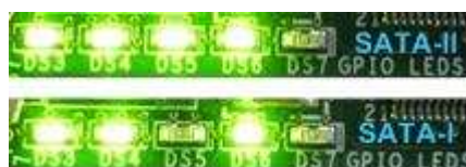
Figure 3 LED status after system set up complete at SATA-II and SATA-I speed
