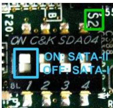
Figure 2 Switch setting on SP605 for SATA-II or SATA-I Host PC
