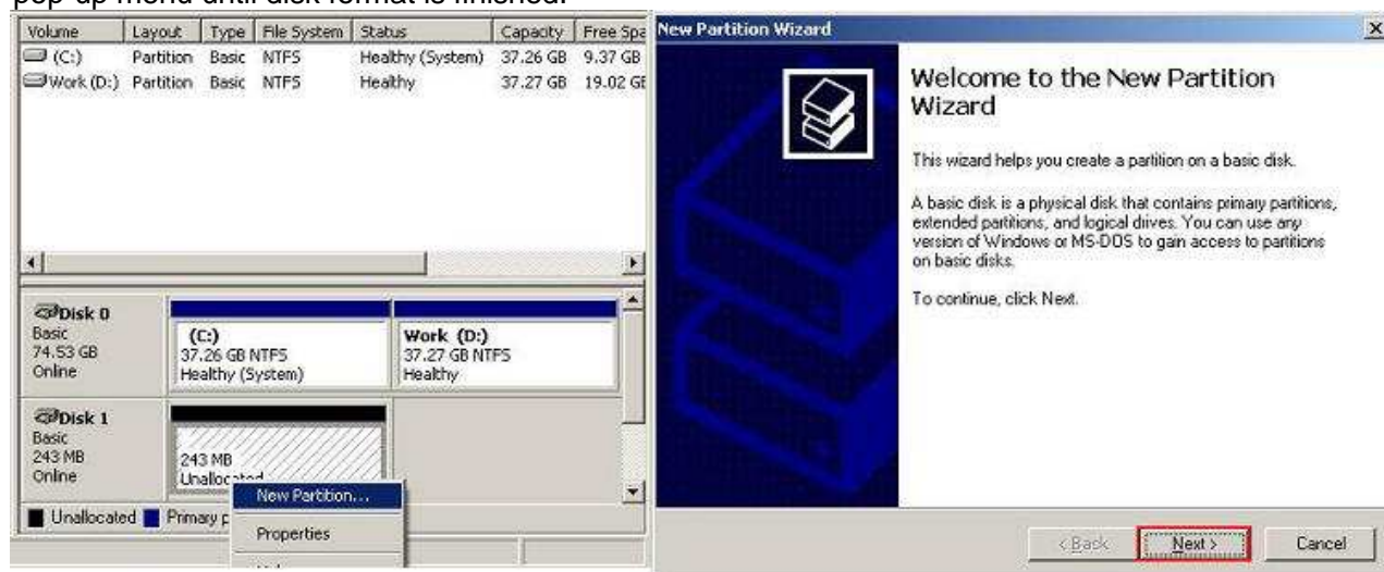
Figure9 Create new partition and format disk
