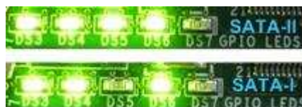
Figure 3 LED status after system set up complete at SATA-II and SATA-I speed
