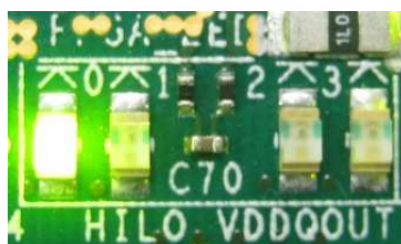
Figure 3-7 LED Status after push StartSW
