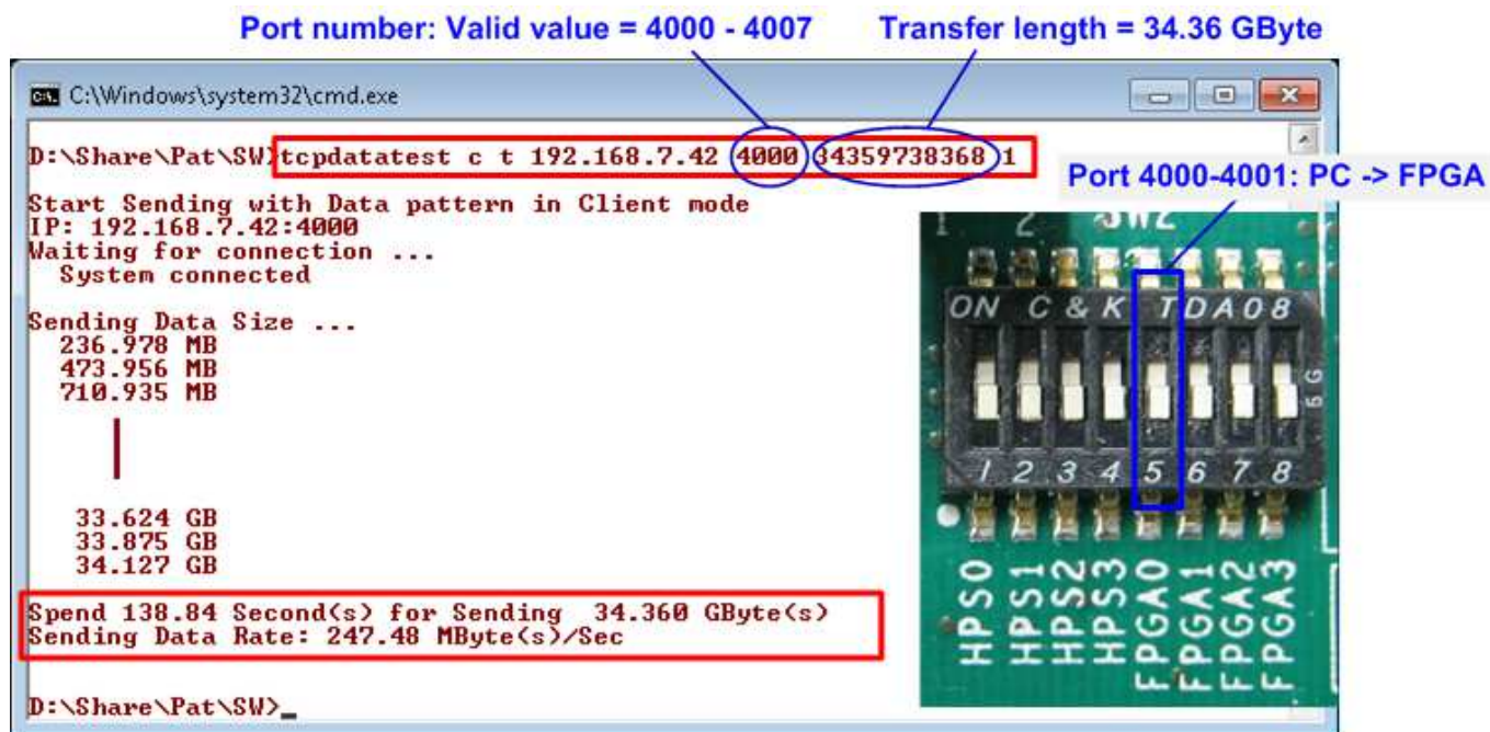
Figure 4-5 Receive data test by using Port#4000 and DIPSW setting
