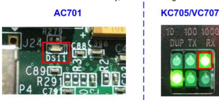
Figure 4-6 Link Status LED from PHY chip
