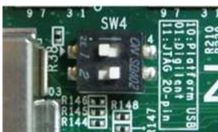
Figure 4-2 SW4 setting to use USB-to-JTAG on ZC706 board
