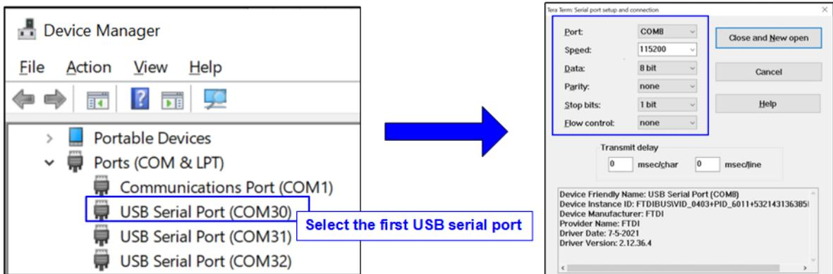
Figure 13 Serial console of the First USB Serial Port
