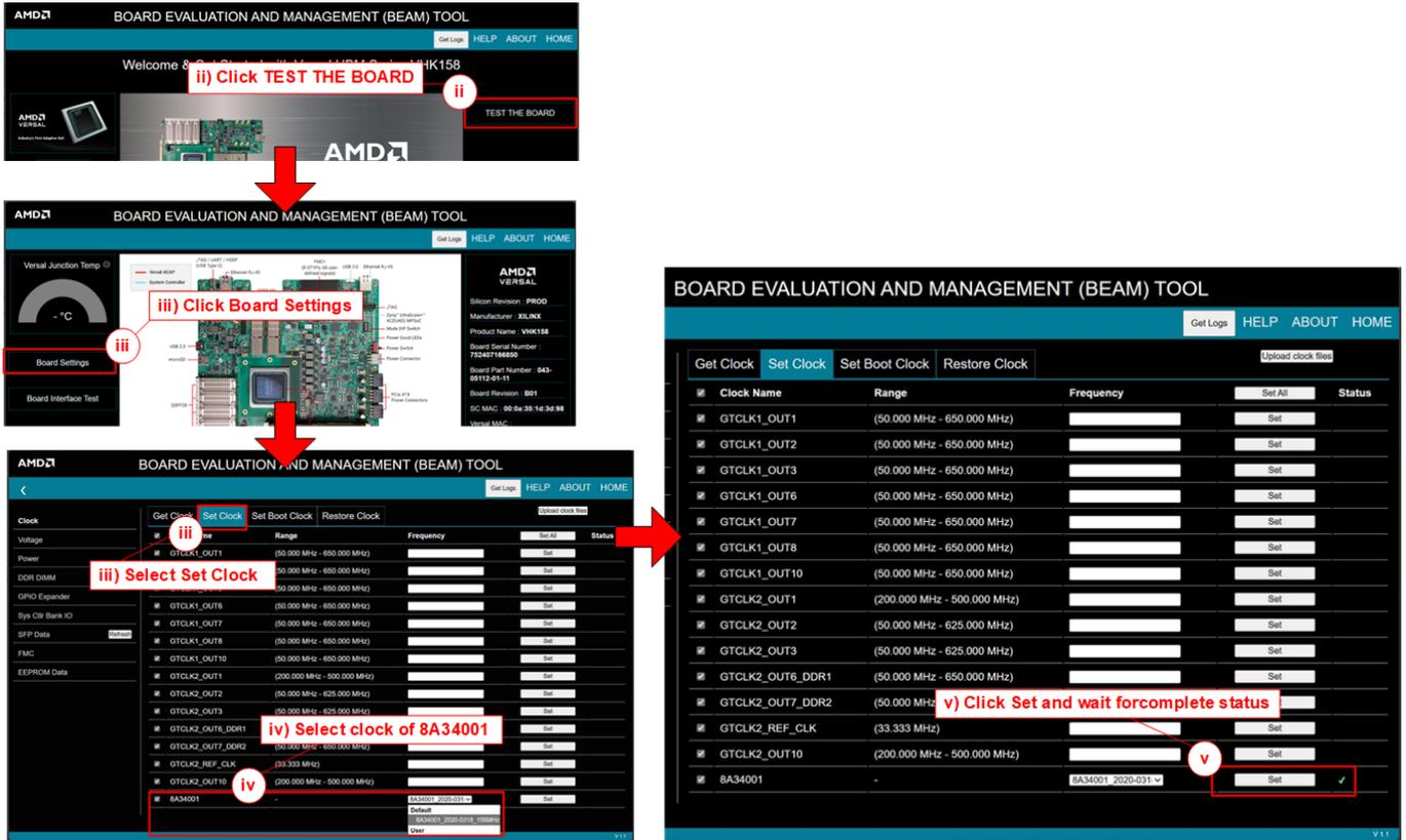
Figure 12 Programmable Clock Configuration for VHK158
