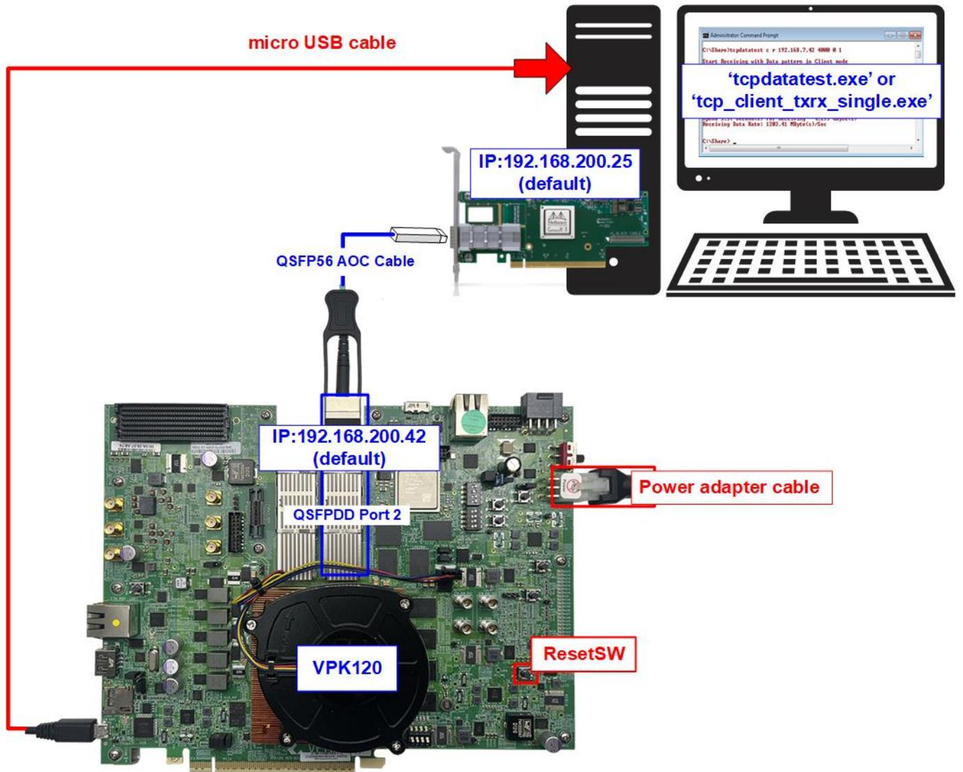
Figure 2 TOE200GADV-IP Demo (FPGA<->PC) on VPK120
