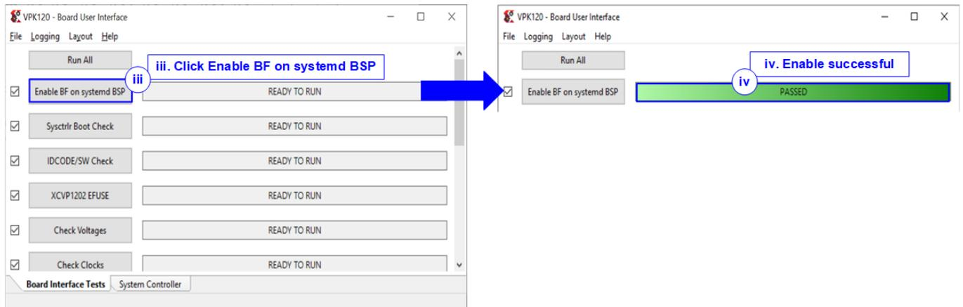
Figure 8 Enable Board Framework on VPK120
