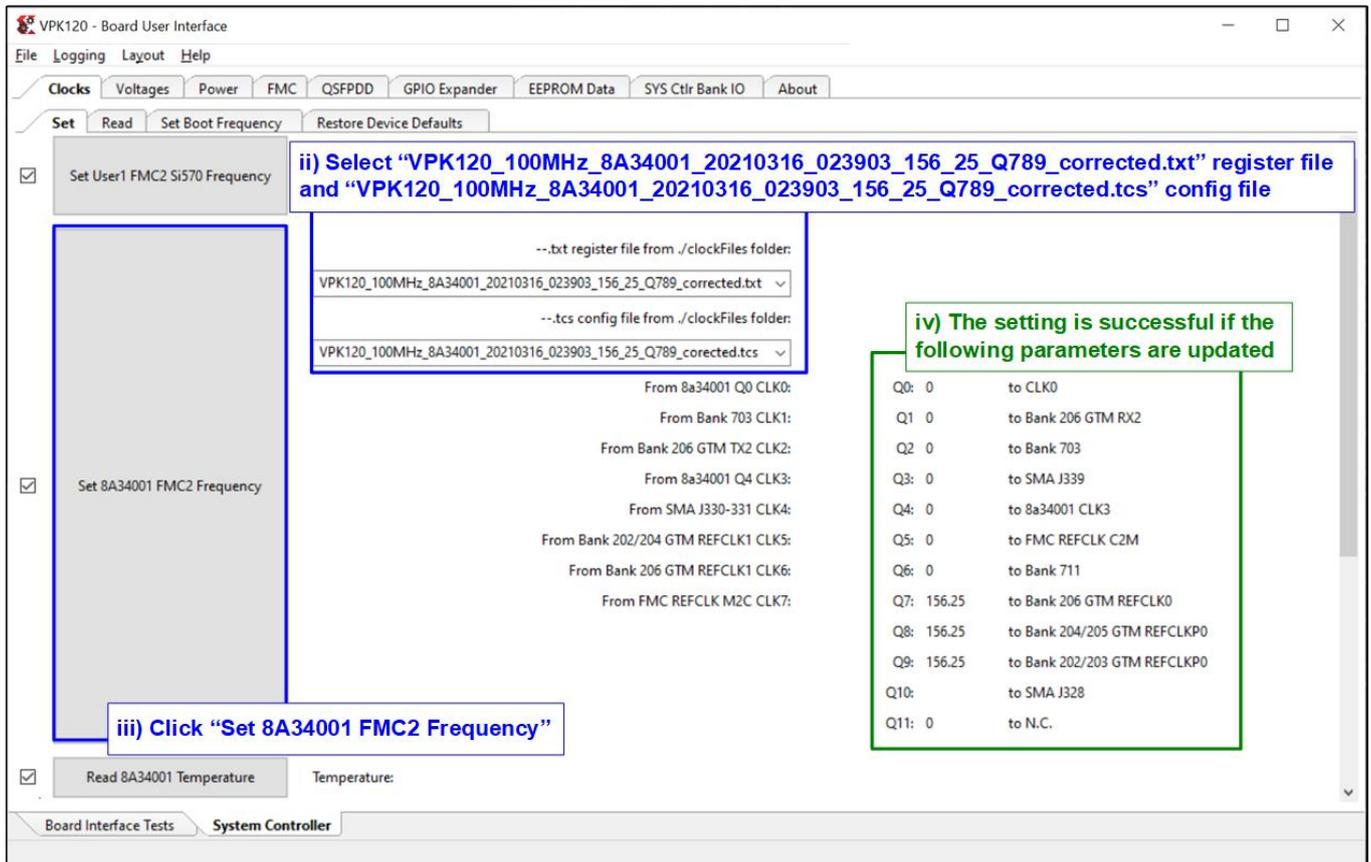
**Figure 10 Reference Clock Programming for VPK120**
