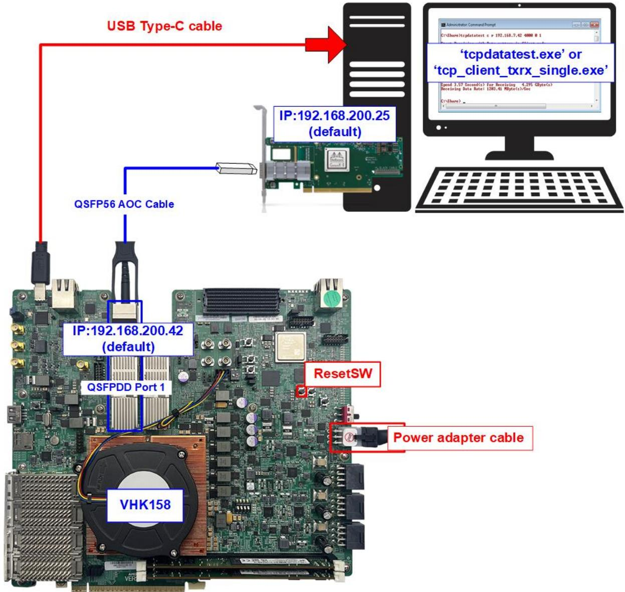
Figure 3 TOE200GADV-IP Demo (FPGA<->PC) on VHK158
