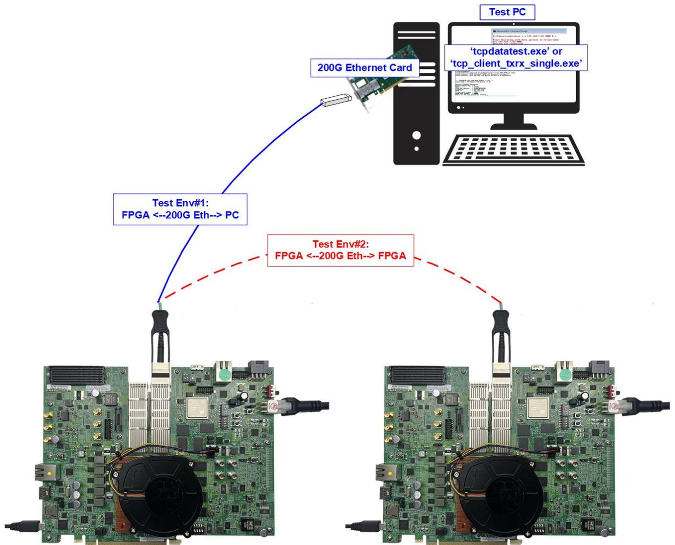
**Figure 1 Test Environment for the Demo**
