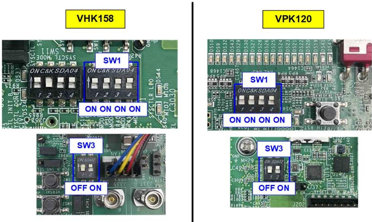
Figure 4 FPGA Board Boot Setting
