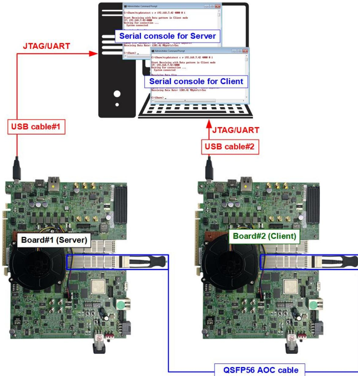
Figure 18 TOE200GADV-IP Demo (FPGA<->FPGA)
