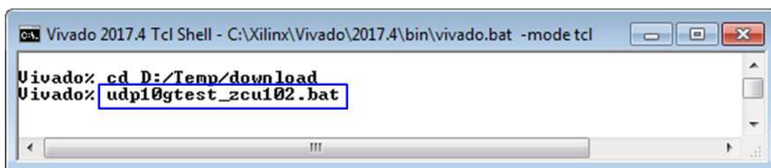
Figure 4-5 Example command script for download to ZCU102 by Vivado tool
