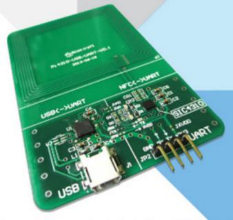
A harvesting module featuring UART or USB interface and two LEDs that can be controlled via GPIO pins. The on-board inductive antenna can generate a current up to 10 mA.
