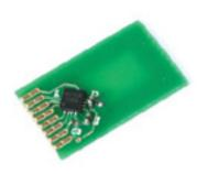
A 12.5 x 19.7 mm tiny module with a UART interface and 4 GPIOs. SIC4310-USB
