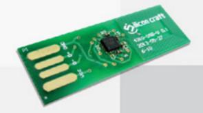
A 12.5 x 37.3 mm tiny module with a USB interface.
