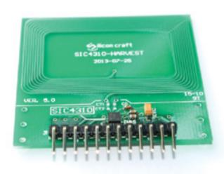
A harvesting module with a UART interface and 3 GPIOs. The on-board inductive antenna can generate a current up to 10 mA.
