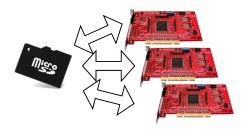
Configuration start by inserting microSD to SDLink even after power up
