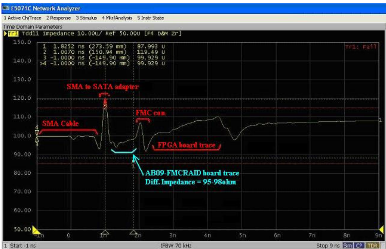
Figure-4: AB09-FMCRAID differential impedance (CH#3) (Measured by Agilent Network Analyzer E5071C)
