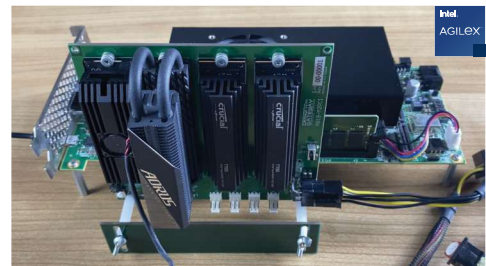
NVMe-IP PCIe Gen5 4ch RAID0 Evaluation on Intel® Agilex™ 7 I-series FPGA Dev Kit
