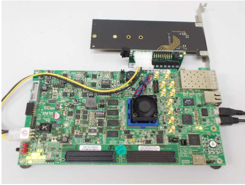
Evaluation on KCU105 with Samsung SSD 960 Pro
