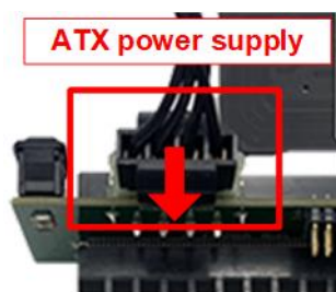
Figure 2-3 Connect ATX power supply to PCIe adapter board
