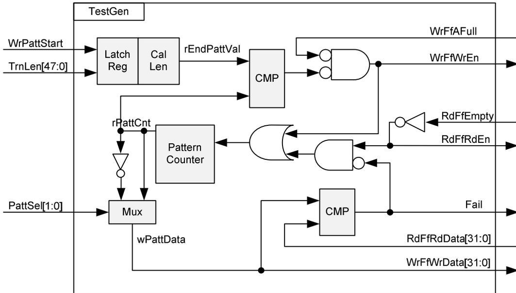
Figure 4 Logic design in TestGen
