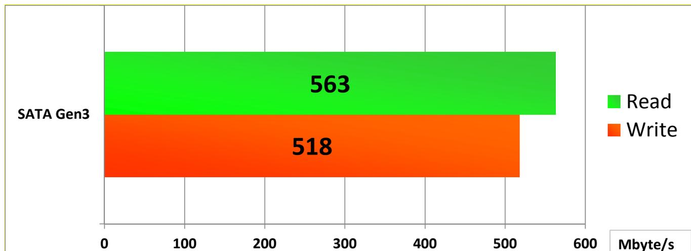
Figure 5-1 Test Performance of SATA Host IP demo by using Samsung 850 Pro SSD
