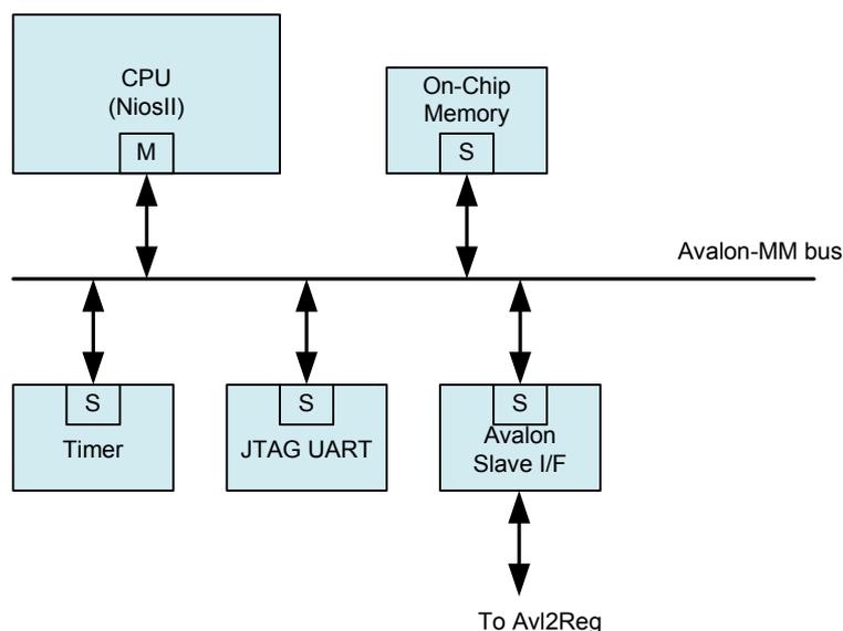
Figure 2-1 CPU system in reference design
