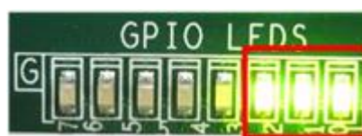
Figure 6 LED status after system set up complete when linkup at SATA-3 speed
