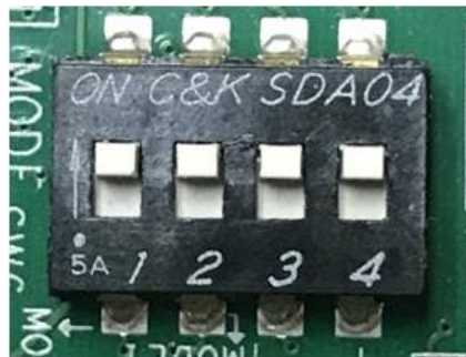
Figure 2-1 SW6 setting to configure PS from JTAG on ZCU102
