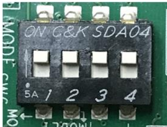
Figure 2-5 SW6 setting to configure PS from JTAG on ZCU102
