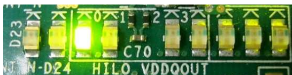
Figure 3-7 LED Status after press StartSW
