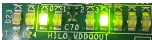
Figure 3-9 LED Status when running Performance Test mode
