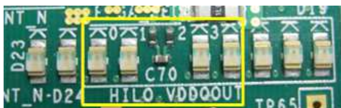
Figure 2-1 FPGA LED to show test status
