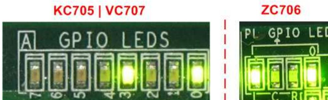
Figure 10 LED Status when running Performance Test mode
