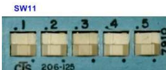
Figure 5 SW11 setting to configure PS from JTAG on ZC706 board
