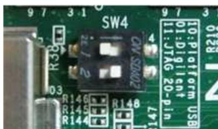
Figure 6 SW4 setting to use USB-to-JTAG on ZC706 board
