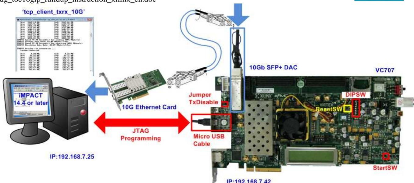
Figure 2 TOE10G-IP Full Duplex Demo Environment Setup on VC707
