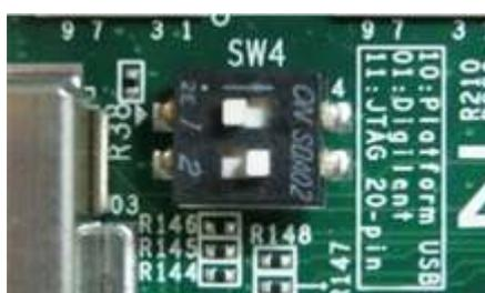
Figure 4 SW4 setting to use USB-to-JTAG on ZC706 board
