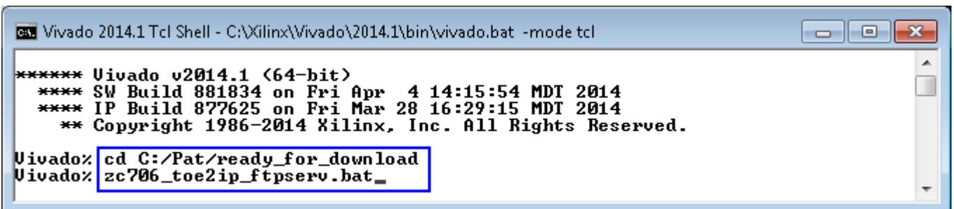
Figure 7 Example command script for download to ZC706 by Vivado tool
